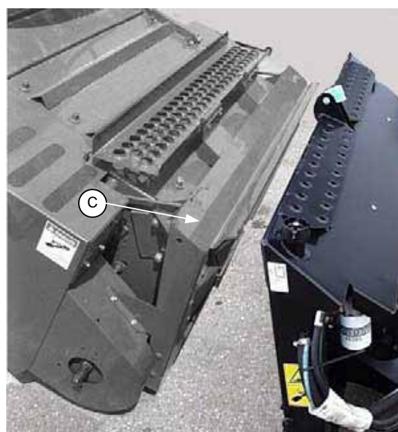
ALIGN FEEDER SADDLE UNDER ADAPTER FRAME
